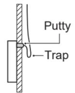
Avoid the water enter into the wired remote controller, use trap and putty to seal the connectors of wires during wiring installation.
