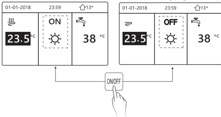
Use the room thermostat to turn on or off the unit for space heating or cooling.
