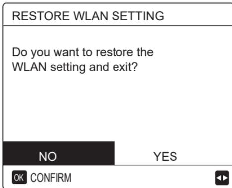
Use "◀", "▶" to move to "YES", press "OK" to restore WLAN setting. Complete the above operation and wireless configuration is reset.
