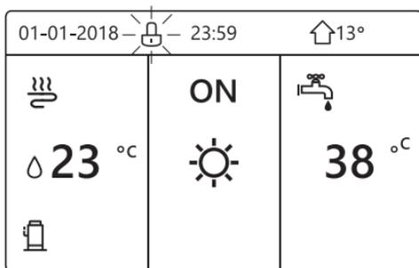
The interface will be locked if there is no handling for a long time (about 120 seconds). If the interface is unlocked, long press "unlock", the interface will be locked.
